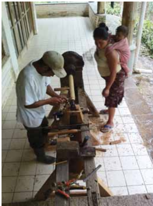
(Below) Beth and company put this lathe in working order on her trip to Guatemala. It's made from an auto differential, with a hand crank, and a tailstock that a colleague made with a chainsaw.
