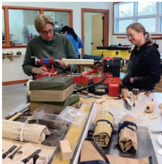
(Below) Beth and company put this lathe in working order on her trip to Guatemala. It's made from an auto differential, with a hand crank, and a tailstock that a colleague made with a chainsaw.
